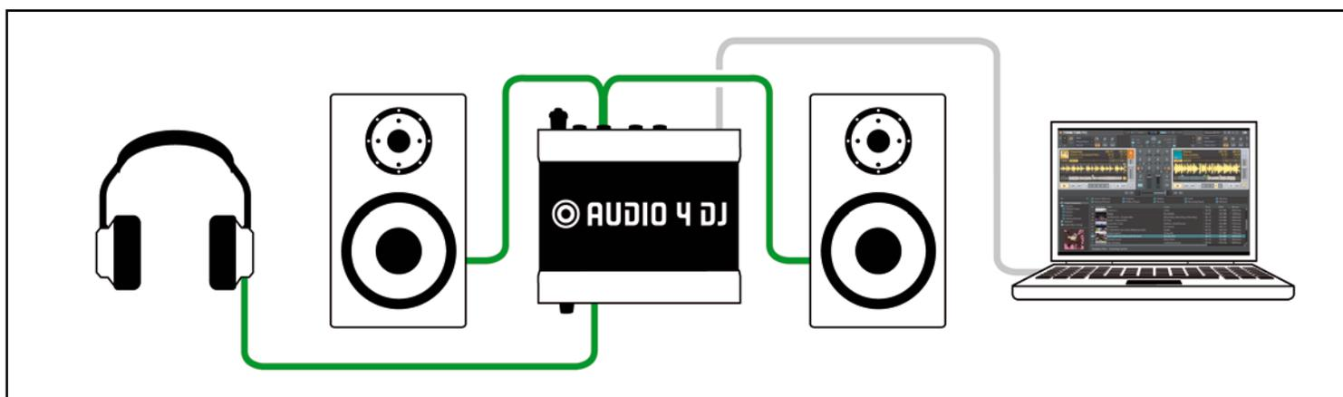
To use the AUDIO 4 DJ for laptop DJing, connect the devices as pictured in the above diagram.
