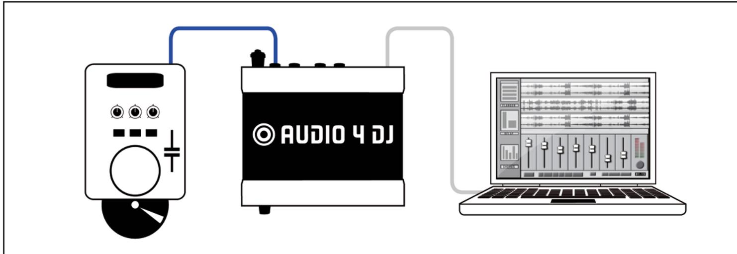
To record audio from an external CD player, connect the devices as pictured in the above diagram.
