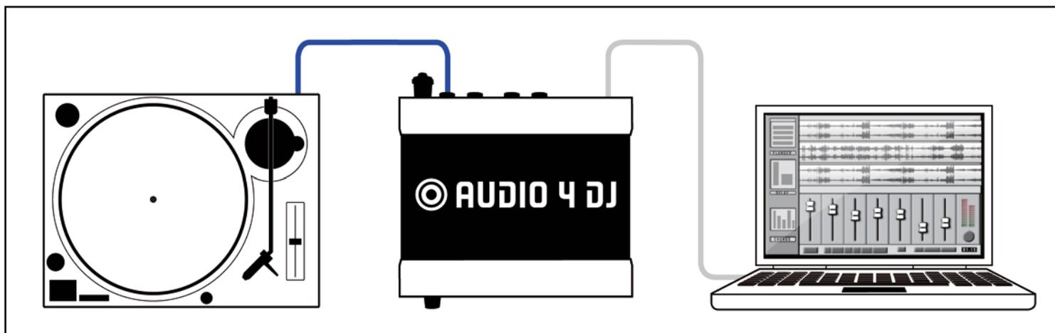
To record audio from a turntable, connect the devices as pictured in the above diagram.
