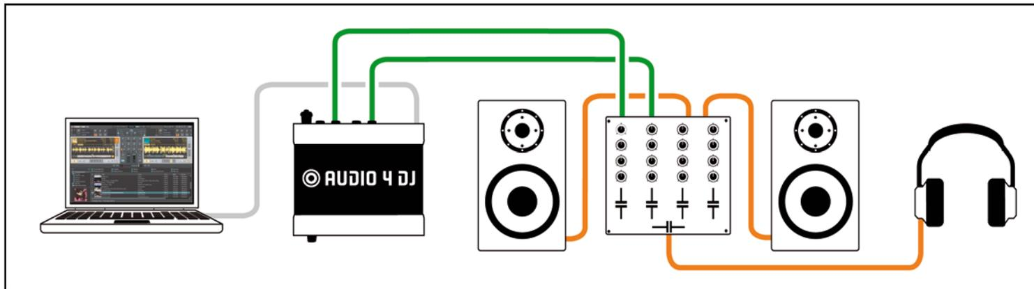
To add a mixer to your DJ setup, connect the devices as pictured in the above diagram.
