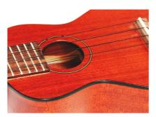
Included in all the other KITs there are water stickers with the image of a soundhole binding. Fixing them is very easy. You only got to put them into soft warm water. Later the binding can be covered with lacquer (photo on the left).
