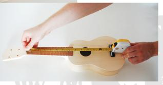
Attention: The distance between the nut and the saddle (which takes place on the bridge) has to be exactly the double like the distance between the inside edge of the nut and the inside edge of the 12. fret (2. Photo on the left side)!!! The bridge itself must also take place in the middle of the top so that the
