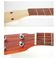
stick out wood parts of the neck on each side of the fretboard with the rasp, file and the different sandpapers. While doing this you should always take care on keeping the shape of the neck organic and round. The neck should also feel very smooth and comfortable after that.
