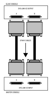
Sys-Link V2 input/output option A blank plate is fitted in both positions as standard. This may be replaced with optional cards which provide the console inputs, outputs and PFL system on pairs of 37way D connectors for linking to other Allen & Heath consoles already fitted with Sys-Link V2. The GL2800 can become an input channel expander (slave) or have its number of input channels expanded (master) when linked to other consoles.
