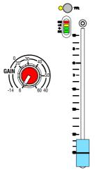
**Mixing with faders or gain controls?** There is a technique used by some operators where they set all the faders to '0' position and balance the mix using the channel gain controls. We do not advise this method as the signal to noise ratio and control resolution can be severely degraded. In addition, it is impossible to mix monitors from FOH in this way as changes to the gain settings affect the monitors too.
