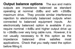
There are two balanced driver ICs which may be used. Either is suitable. These are available from Allen & Heath or good electronic component suppliers. The Allen & Heath part number is shown below:
