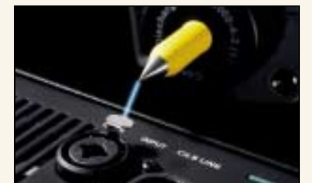
Lab.gruppen's EMC test facilities. 8,000 volts are being "shot" with this gun for testing!
