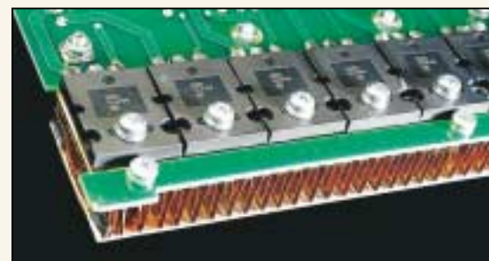
The output transistors are located side-by-side in the airstream.
