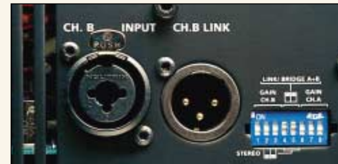
Neutrik Combo® input jacks adapt to both worlds, XLR or 1/4” phone plugs.
