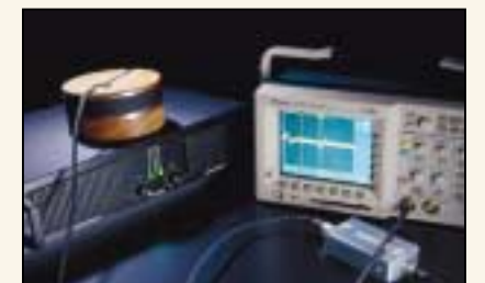
The very finest test equipment is made in-house; here is a coil for measuring the hum field.
