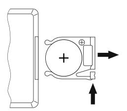
Insert the battery into the remote
