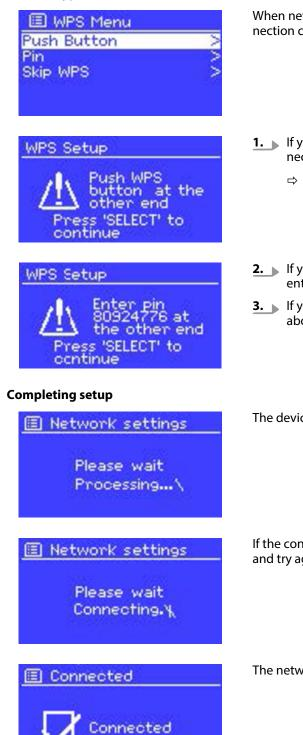
When networks are WPS-encrypted, the network name begins with WPS. The connection can be made in three different ways:
