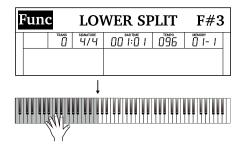
This feature allows you to select a point that splits the entire keyboard into two sections and to assign different sounds to those sections. The preset split point is on piano key [F#3].
