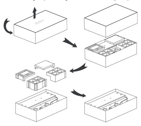
Place the box upside down on a suitable surface, open the box and remove the foam protection.
