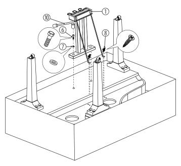
Carefully turn the pedal unit (1) over and fasten it to the keydesk with two of the supplied washers (7) and hexagonal screws (6) using the hexagonal screwdriver (10) and four of the supplied screws (8) as shown.
