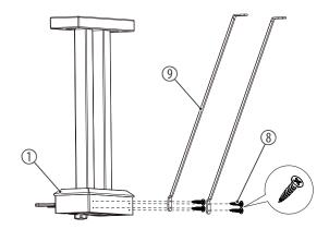
Attach the supports for the pedal unit (9) to the pedal unit (1) using two of the supplied screws (8) each as shown.
