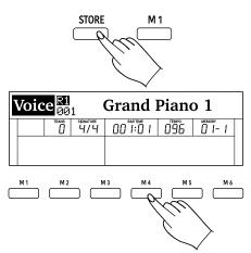
Hold down [STORE] and press one of the [M1]...[M6] buttons to save the current settings in the respective memory location (M1 to M6).
