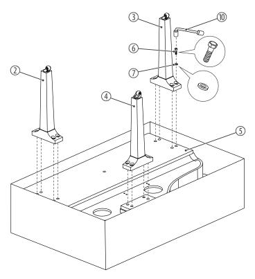
One after the other, screw the three supports with each four of the supplied washers (7) and hexagonal screws (6) using the hexagonal screwdriver (10) as shown on the underside of the keydesk (5).
