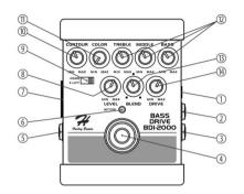
1 Connector for external power supply, e.g. a 9 V AC/DC adapter. If this connection is used, the battery is automatically disconnected from the circuitry.
