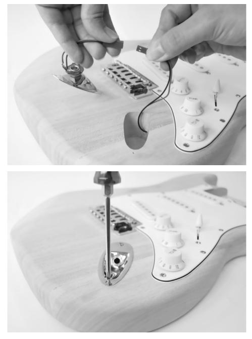
Now connect the connector for the output jack socket to the connector for the pickup and the potentiometers. Insert the output jack socket into the hole provided on the body's front side and screw it in place using the screws provided.
