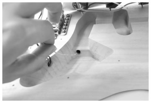
Thread the cable for the string earthing (after stripping the insulation, and without the connector) to the spring claw through the recess in the opening on the back.
