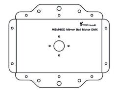
When installed, the motor axis must be exactly perpendicular to the ceiling level!
