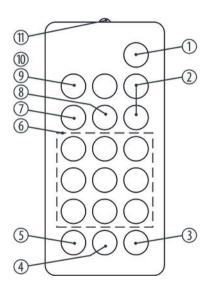
To use the remote control, point it with the infrared diode to the infrared sensor on the unit and press the desired buttons. The maximum distance from the unit is about 9 m. The device will only respond to the remote control signals if it is not controlled via DMX.
