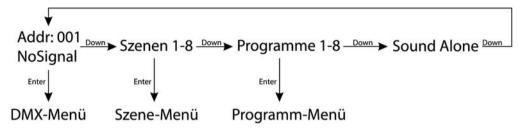
Press repeatedly [DOWN] while 'A001' is flashing in the display to call one of 8 preprogrammed scenes, one of 8 programmes or to set the device to sound-controlled mode.
