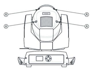
**16.** Put the upper part of the housing back on the base. At that point, both housing parts must engage in the circumferential seal profile. Replace the four Phillips screws ('A') to the top of the housing and tighten them.
