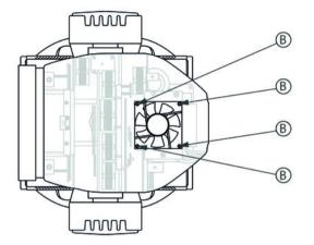
**15.** Reattach the fan and secure it with the two Allen screws (marked in the illustration by 'B'). Make sure that this also secures the heat shield.
