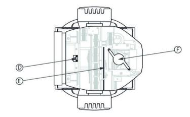
**8.** Remove the heat shield located under the fan ('F').
