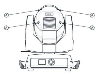
**3.** Open the housing by unscrewing the four Phillips top screws marked in the illustration above by 'A' and remove the upper part of the housing. Make sure that no screw falls inside the unit.
