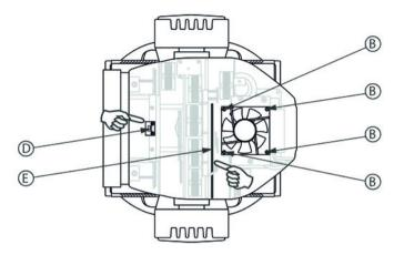
**4.** Check that you have removed the proper cover. Compare the exposed interior of the unit with the illustration. If you can see the heat sensor (marked in the illustration by 'D') at this point, the proper side of the case has been opened. If the correct side of the case is open, you can also clearly see the colour wheel (in the figure marked by 'E').
