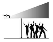
In order to meet the limits for maximum irradiation (MZB limit value for the non-hazardous irradiation of the eye or the skin with a laser), the device must be installed at a height of at least 2.7 m according to the BGV-B2 valid in Germany.
