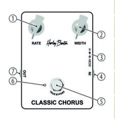
1 **RATE**Turn this control clockwise to increase the speed of the effect.
