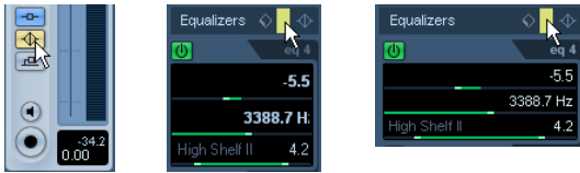
EQ bypass in the mixer, the Channel Settings window and the Inspector
