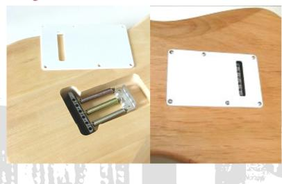
This cover has to be adjusted very well in its place (second photo on the left) so that you can put in strings later on while changing them - without unfixing the plate again. The holes have to be drilled - and at all the cover is the best way having a fine template to mark them!! After drilling the plate has to be fixed with its wood screws. No problem at all I think.
