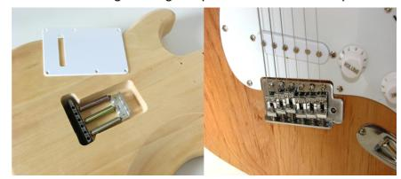
vibrato unit by hooking them in. Take care and don't get the two screws too much into the wood. This is important for adjusting the whole thing later on after the guitar got stringed and tuned.
