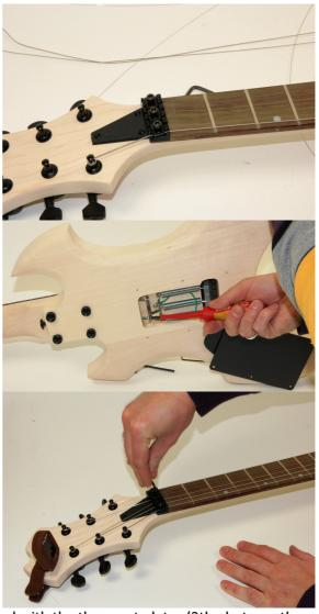
And now strings can be fixed with the three nut plates (3th photo on the left side above). All six strings can be fine tuned yet with their tuners at the end of the tailbridge unit (2nd photo on the left side).
