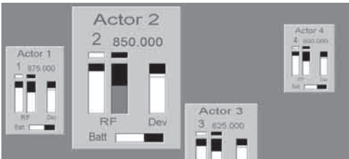
Fig. 2: Display of a scene configuration with four actors on the S-MCD Mikroport computer display
