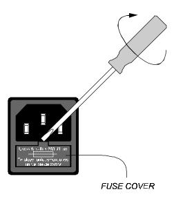
Use a small flat screwdriver as shown to slide the fuse cover out from the power inlet module. The fuse can be found inside the fuse cover module after it is pulled out.
