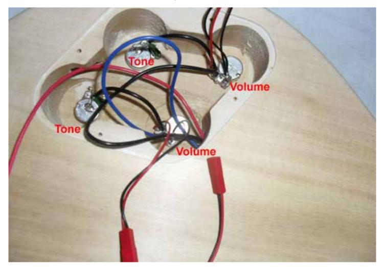
Take out the cable without connector (ground wire) and insert it into the pre-drilled bridge hole through the channel. Just leave it in the bridge hole. It will connect to earth when the boots of the bridge are pressed on it.
