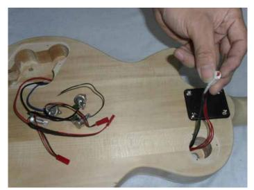
Then put the potentiometers on the right positions as shown in the following picture. The Tone and Volume potentiometers on the downside should be connected to the neck pickup. The Tone and Volume potentiometer on the upper side should be connected to the bridge pickup.
