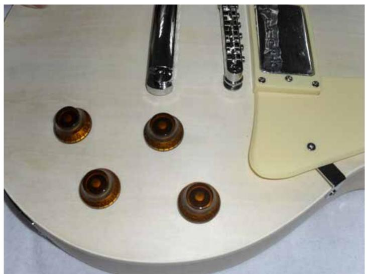
Put the knob on the shaft of each potentiometer.
