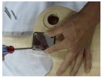
Turn the assembly over and position the neck plate (with its black protective seal) over the four bolt holes at the rear of the body and drive in the four long screws through the neck plate, body and pilot holes in the neck until all fits tightly.
