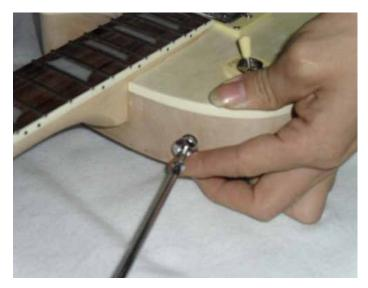
Screw the strap buttons into the pre-drilled holes at the bottom edge of the body and at the top next to the switch.
