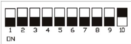
Set DIP-Switch 10 to ON in order to determine the Slave device.
