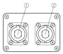
1, 2 NL4 connections, wired in parallel (INPUT, THRU)
