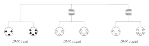
DMX OUT: connect the DMX receiving device(s) here DMX IN: connect the DMX transmitting device here
