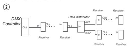
You can run a maximum of 32 units (receiver) per output channel. Use a terminator on the last receiver.
