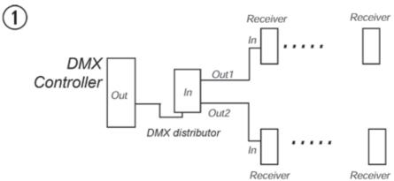
You can run a maximum of 32 units (receiver) per output channel. Use a terminator on the last receiver.
