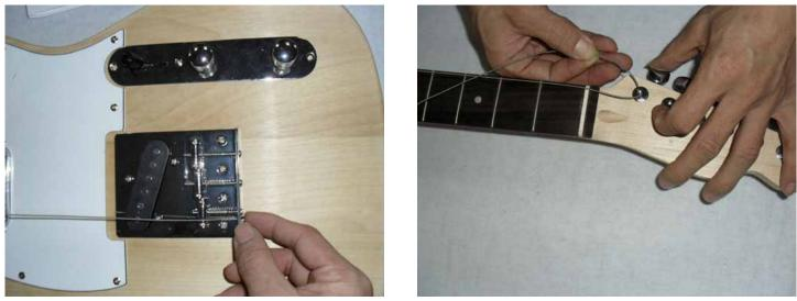
Ensure that the string sits smoothly on its saddle and keep taut whilst winding a couple of turns on the relevant tuner. Thread through the string post and bend the string back on itself to anchor it in place. Apply a little tension from the tuner and move on to the next string. Repeat the above process for all six strings.
