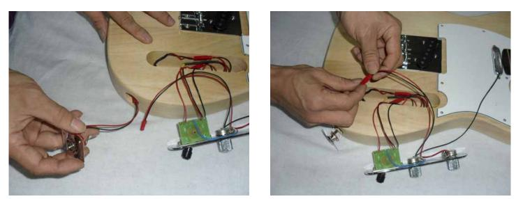
Gently thread the cable on the potentiometers lead through the hole behind the tone control cavity to the separate routing for the jack socket. Connect the connector wire to the connector on the jack socket (they only fit one way round), then fit the jack socket plate and secure it with dome-head screws.
