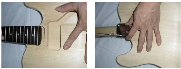
Turn the assembly over and position the neck plate (with its black protective seal) over the four bolt holes at the rear of the body and drive in the four long screws through the neck plate, body and pilot holes in the neck until all fits tightly.
