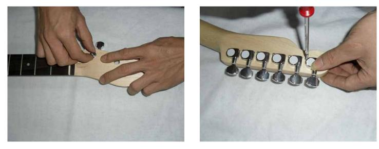
Fix the retaining screw through the loop on the rear of the gear housing into the pilot hole to hold the tuner in position. Then tighten the nut on the front face of the tuner until it is firm by using a spanner of the correct size. Repeat this for the remaining five tuners and then fit the string tree.
