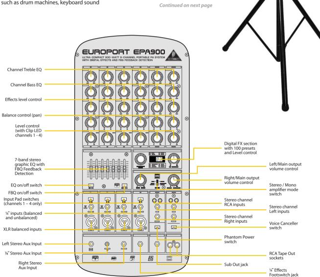
unit on a tabletop and deploy the speakers. Connect the high-quality dynamic microphone and hit the power switch—voilá, instant PA system! There is even an onboard storage compartment for the included microphone, accessories and cables. And if you need to add some serious bottom-end to your system, just connect an active subwoofer to the handy Sub Out jack.
